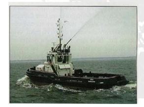
Consequently the very good experience with tugboat TYTAN and TAURUS have led to order for 2 azimuth thrusters to be installed on board of the third in Poland ASD tugboat URAN for operation in Szczecin-Swinoujscie harbour under the Port-Hol owner, starting in Sept. 2001.
